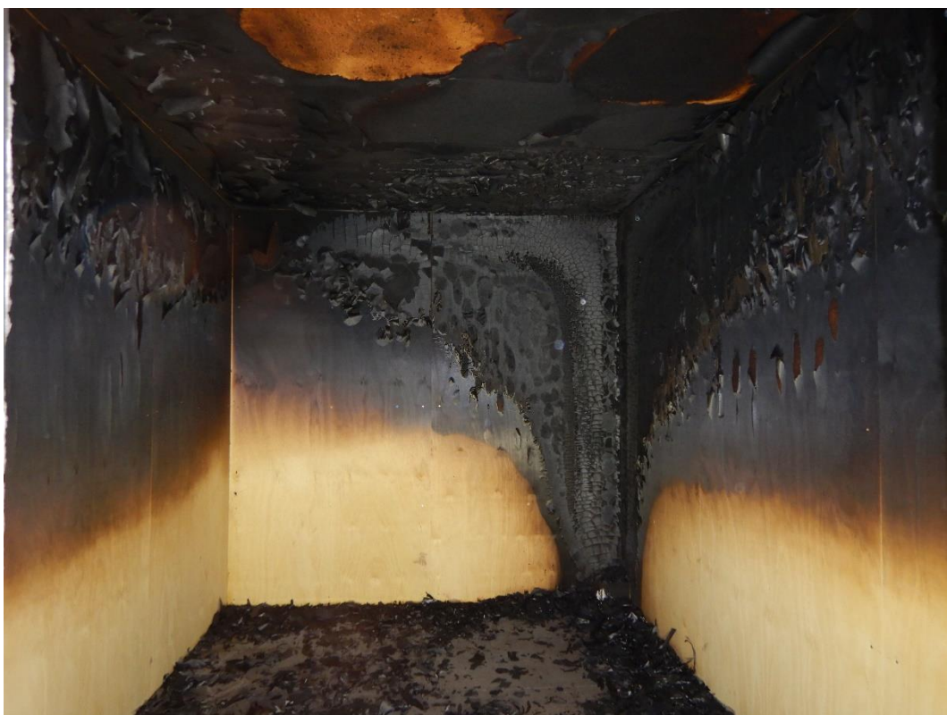
Figure 21 The specimen after the reaction to fire test
