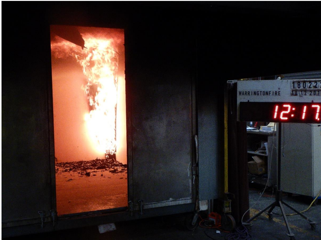
Figure 18 Specimen 17 seconds after burner output was increased to 300kW.
