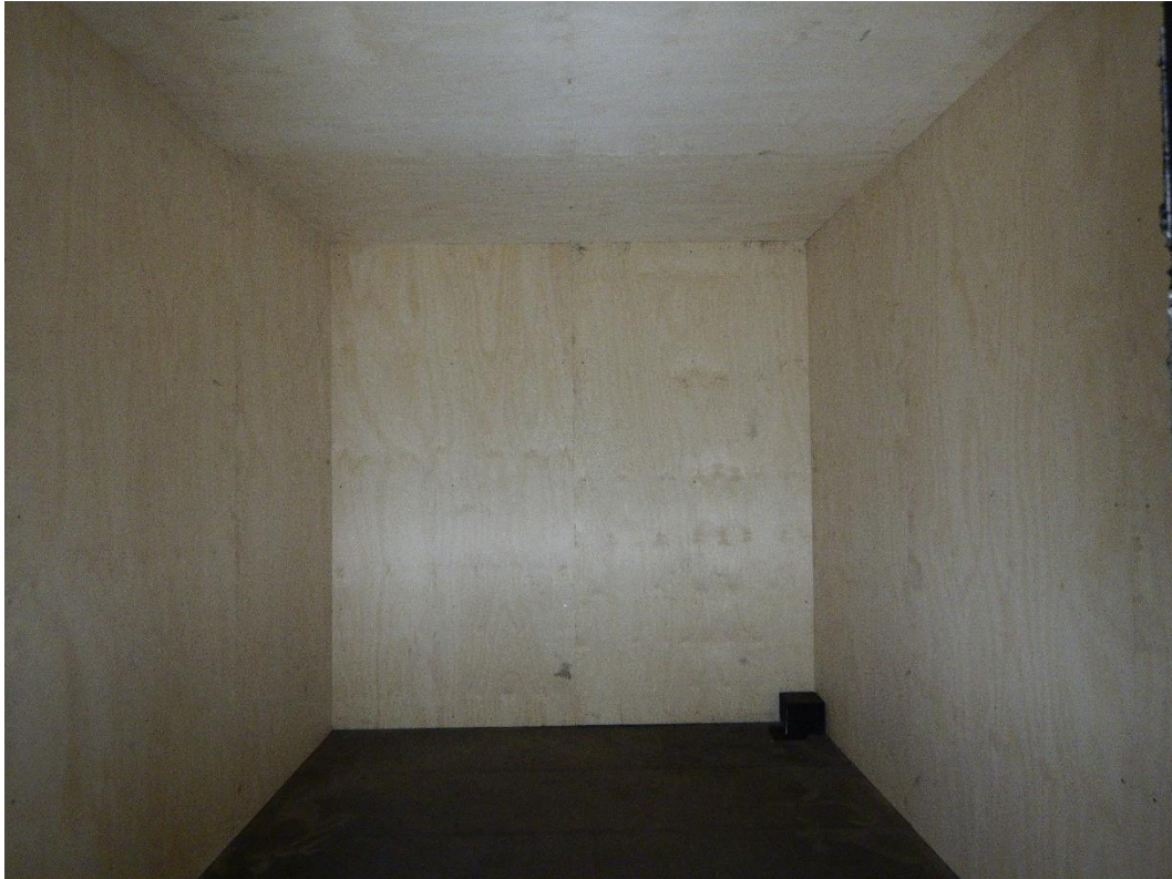
Figure 12 The specimen before commencement of the reaction to fire test
