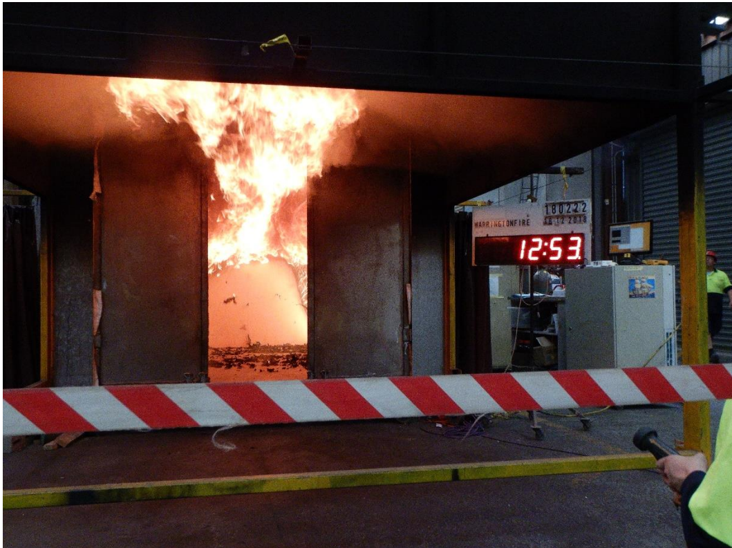
Figure 20 Specimen at the end of the reaction to fire test.
