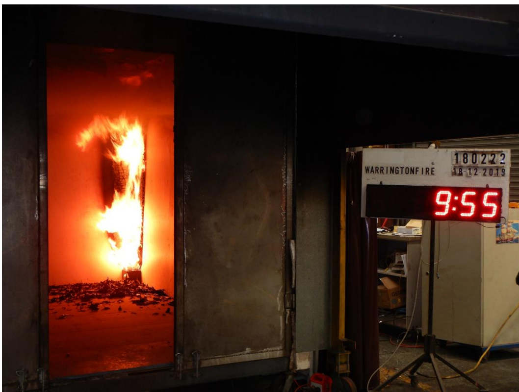
Figure 17 Specimen 7 minute and 55 seconds after ignition of burner.
