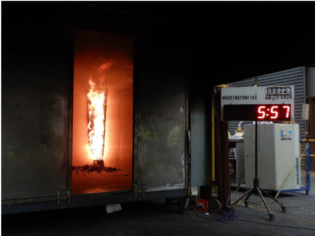
Figure 16 Specimen 3 minute and 57 seconds after ignition of burner.
