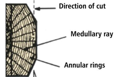
**Crown/Flat Cut** sliced veneer is cut tangentially to the grain. It displays an attractive figure of bold sweeping 'cathedral' curves and oval along the centre of the leaf, with striped grain nearer the edges.
