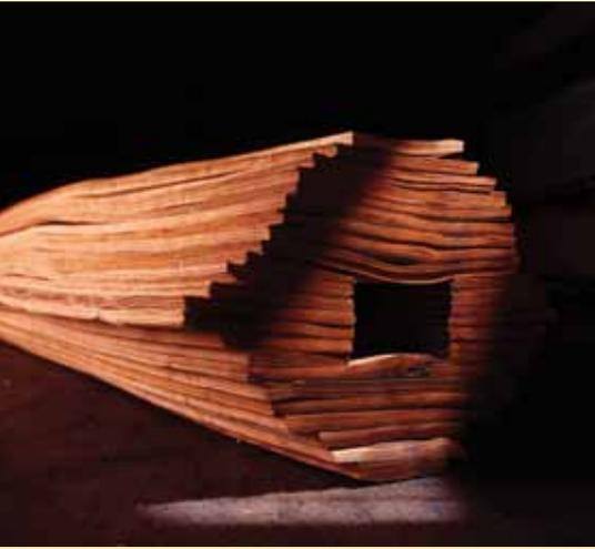
*Veneer sliced and assembled in the shape of the log from which it came.*
