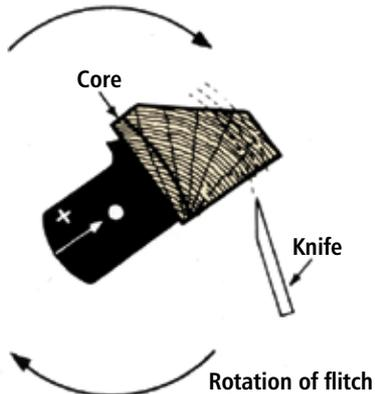
**Rift Cut** is a variation on the quarter cut appearance specifically used to eliminate medullary ray in white and red oak, which results in a broader stripe.
