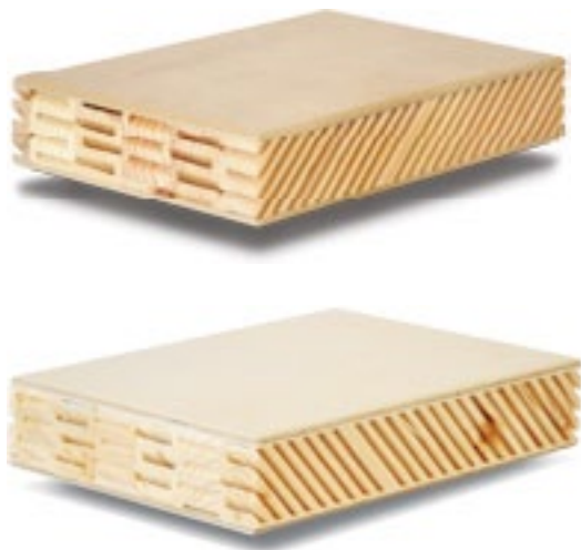
Figure 19: DendroLight® 3-layer furniture panels with (top) MDF faces and (bottom) plywood faces
