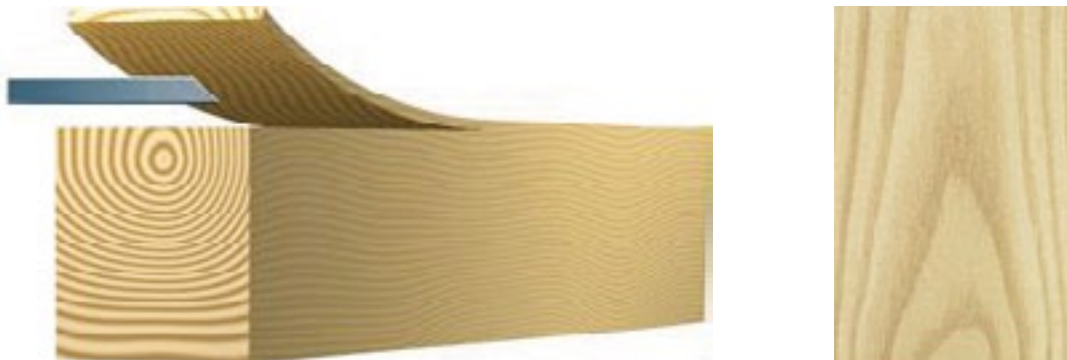
Figure 6: Lengthwise slicing of veneer
