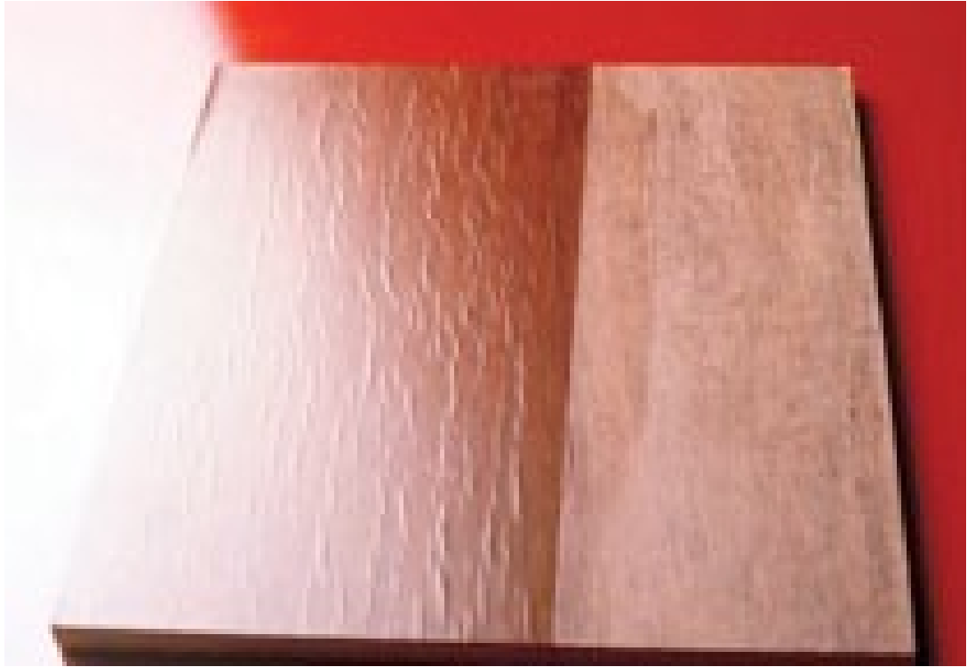
Figure 42: Example of checks developed on veneer surface Source: Barbara Ozarska
